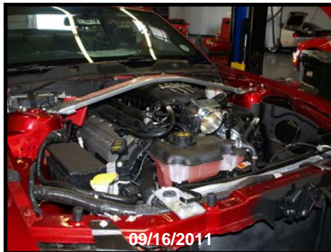
Above, left to right: Rear SMS seats were installed, Boss 302 intake was installed, and the front fascia and hood were removed.
