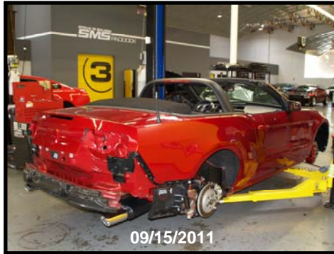
Above, left to right: SMS brakes and suspension were installed, rear fascia and the seats were removed and waiting for the SMS parts.
