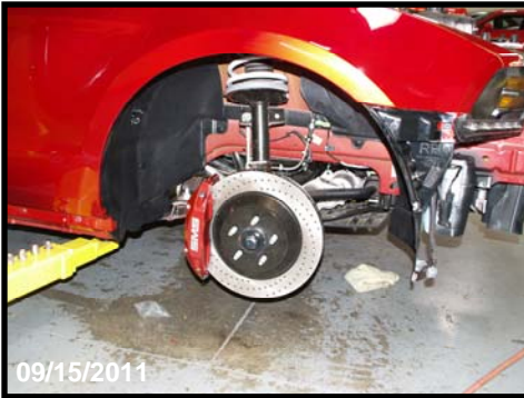
Above, left to right: SMS brakes and suspension were installed, rear fascia and the seats were removed and waiting for the SMS parts.
