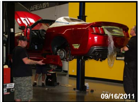
Above, left to right: Front Dual Side Heat Extraction Hood with Chrome Trim and SMS Rear Fascia with Dual Exhaust Cooling Vents, SMS Front Fascia and Blade Front Grille, and the SMS Side Skirts with Integrated Brake Intakes were all installed.
