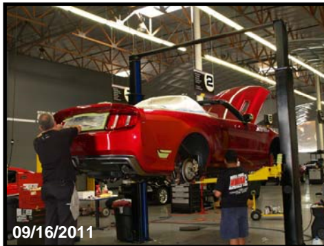
Above, left to right: Front Dual Side Heat Extraction Hood with Chrome Trim and SMS Rear Fascia with Dual Exhaust Cooling Vents, SMS Front Fascia and Blade Front Grille, and the SMS Side Skirts with Integrated Brake Intakes were all installed.
